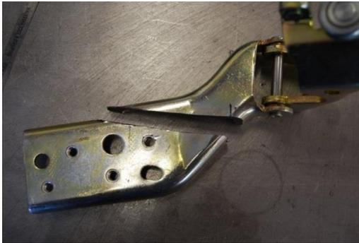
I also cut away some of the excess at this point and I make a small relief cut in the top piece and bend it into the shape of the base.
