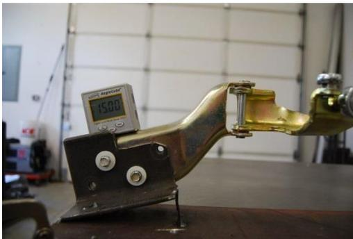
Make note of the distance from the table surface to the top surface of the hinge base. This one is just under 6" for example.
