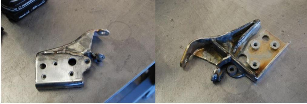
One note about welding these... the more of the cad plating you can get off, the better it is going to weld.
